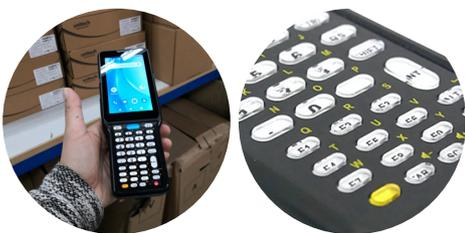
Keypad with backlight design. Durable keypad with 2.5 million lifetime clicks. Hard silicon material with key printing underneath keys.
