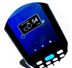
Easily change the HT730 battery without interruption / rebooting the device. Reboot within 1 minute - screen will automatically start the countdown.
